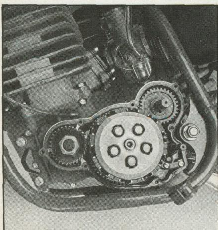
**Geared primary drive, coil-spring clutch**
