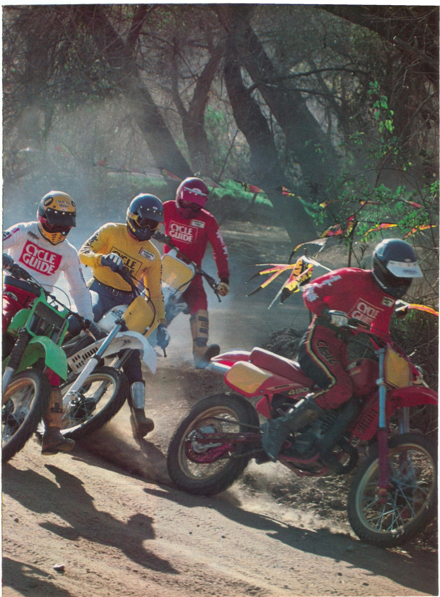
the small, choppy bump instead. And it's there that the Honda's fork and Pro-Link rear end outshine the rest, with the Husky and the Suzuki next in line. But while the RM's rear end is on par with the Honda's, its fork often suffers from a case of the jitters that contributes to the aforementioned high-speed head-nod. By switching from 5-weight to 10-weight fork oil and using the lightest compression-damping setting, the nod was reduced, though not always eliminated.
