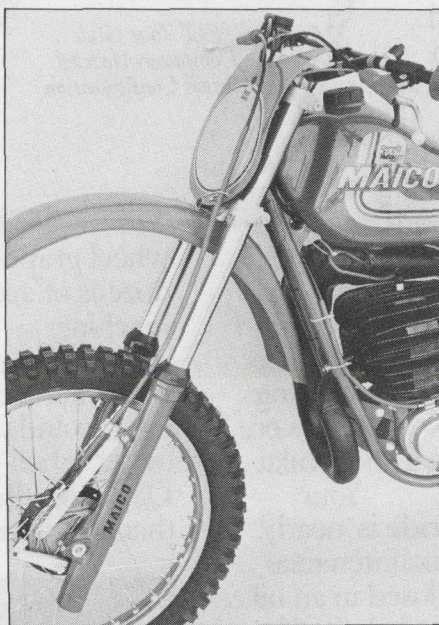
Forks are shorter and have new damping. Front of bike sits lower this year. Wheel travel is 12.2 in.
