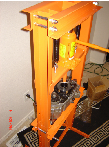
Using a press to compress the Maico clutch to install the circular locking
