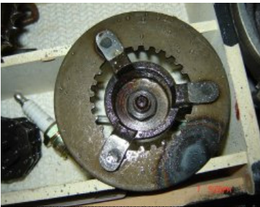
Bottom of the clutch 'Guide' which houses the spring washers with the
